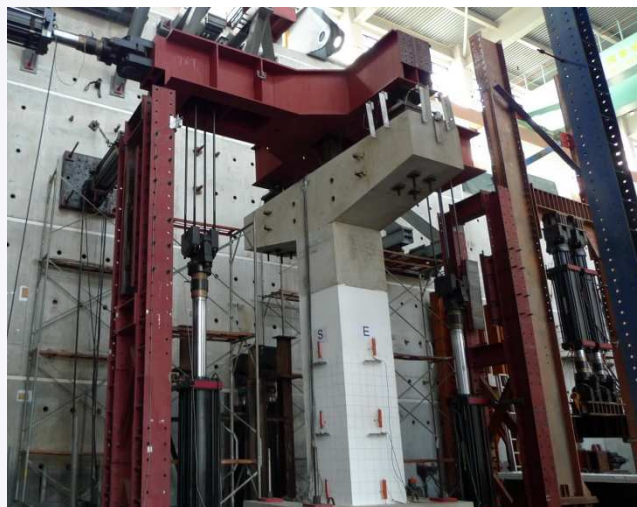
預鑄節塊隔震橋柱之單向反覆載重與擬動態試驗
